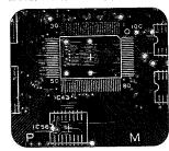
The lines on circuit boards are made of metal and carry electricity. The lines must not touch each other or the electricity will flow to the wrong place, creating a short circuit.
